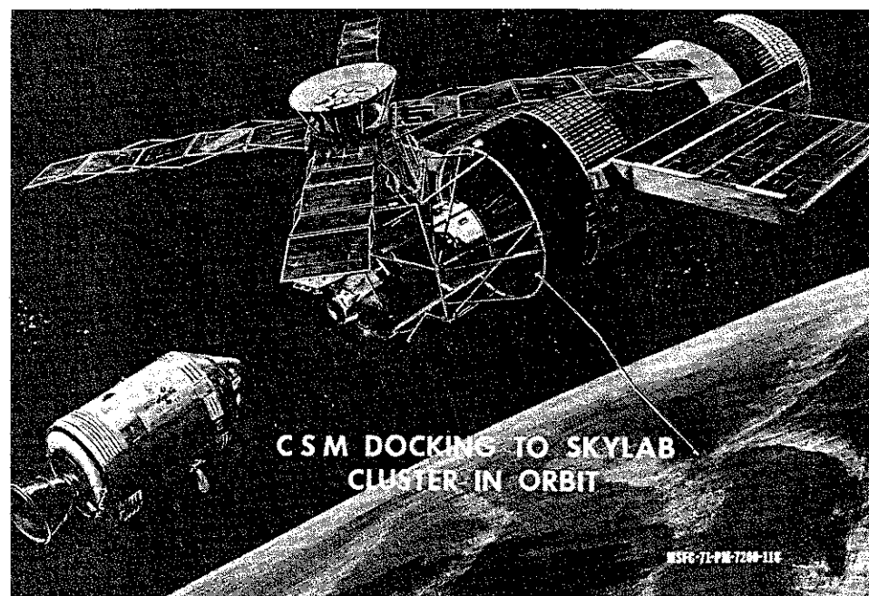
2. Figure 2. Solar panels for Skylab generating about 25,000 watts.
